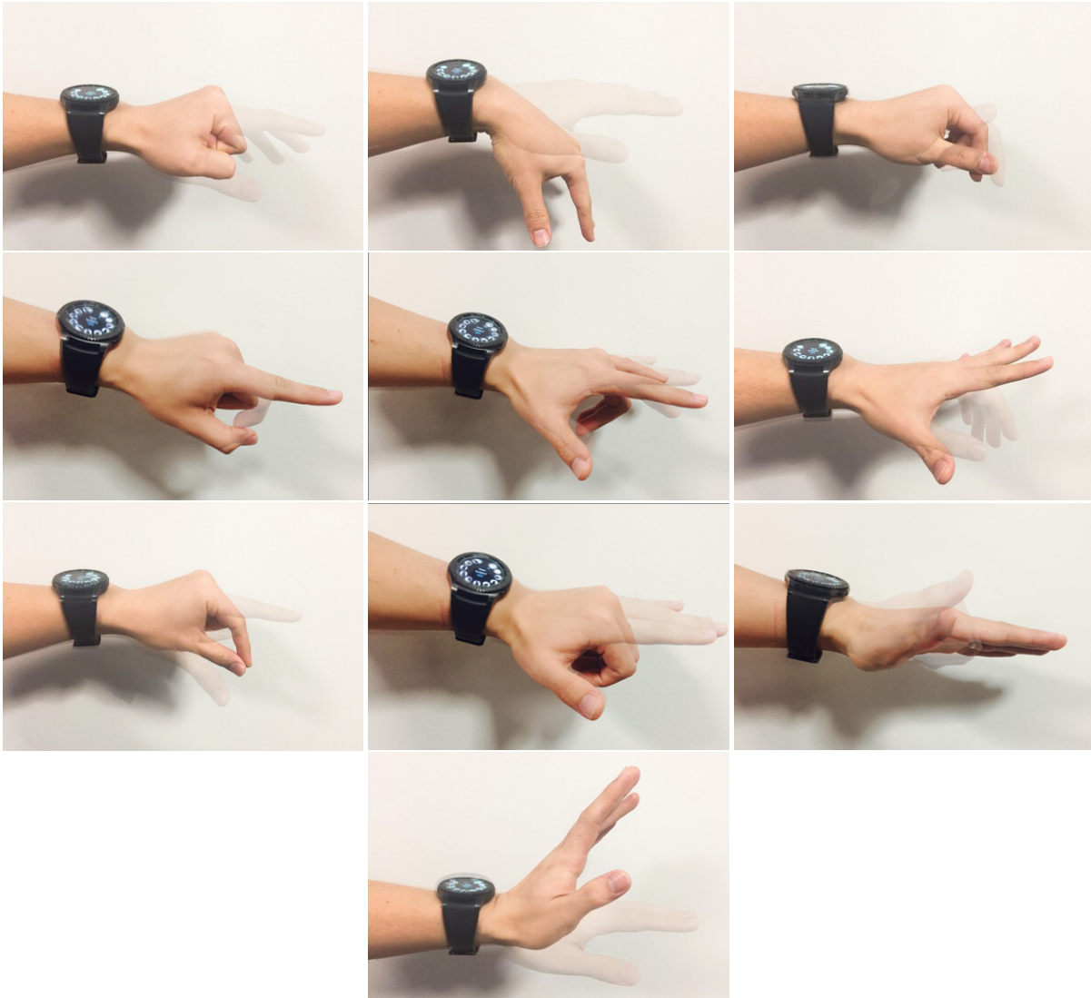
Fig. 4. The conflict-free gestures detected by our system (top-left to bottom-right): Close Hand, Down Hand, Down Rub Finger, Index Flicking, Middle and Ring Clicking, Open Hand, Pinch Fingers, Pull 4 Fingers, Push 4 Fingers, and Up Hand.
