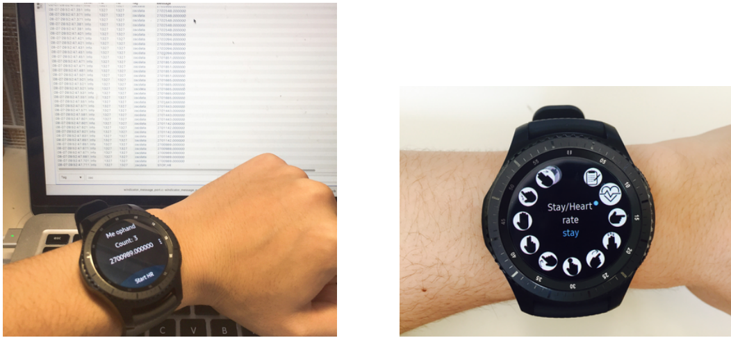
(a) An on-line data application implementation, which requires connection to a host computer for receiving data in real-time via TCP. (b) Implemented for off-line data collection, which offers a local data storage for efficiently collecting data.
