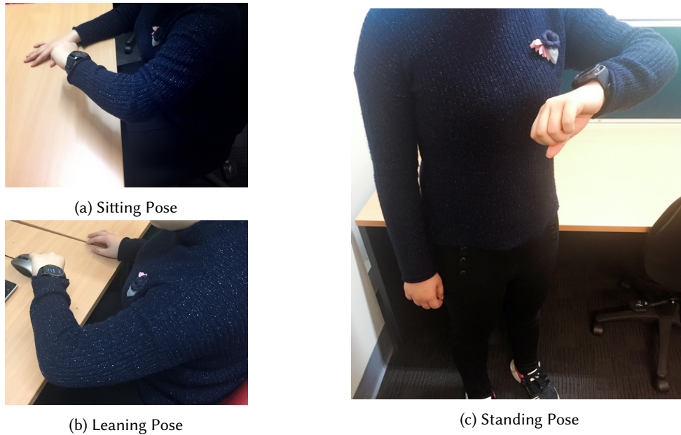
Fig. 15. Three regular use circumstances with different poses of the smartwatch, including: Sit, Sit with the forearm leaning on a table, and Stand.
